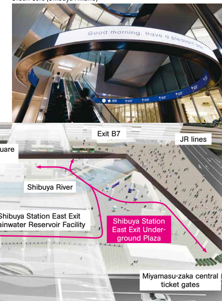
Flow of movement through the Shibuya Station East Exit Underground Plaza
